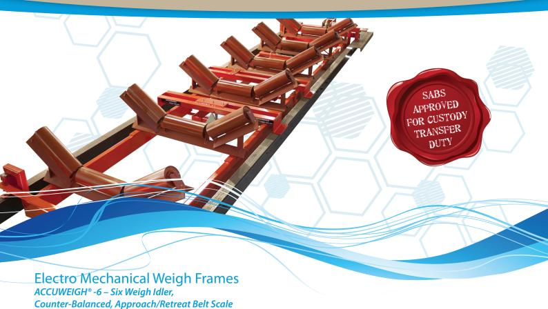
This model incorporates a low deflection, rugged, counter-balanced, six weigh idler, Approach/Retreat weigh bridge design with a single, precision load cell, operating in tension, to provide superior weighing performance over extended periods with minimum maintenance. The load sensor assembly on Accuweigh® weigh bridges is protected against mechanical shock. (Overload protection optional)
